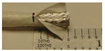
Figure 10: Slitting the cable jacket
