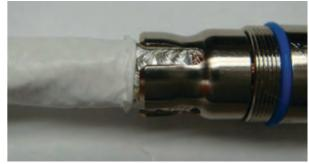
Figure 23: Trimming the outer jacket
