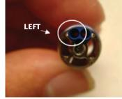
*Figure 19: Inserting contacts into housing*
