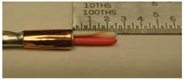
Figure 14: Removing the foil edge
