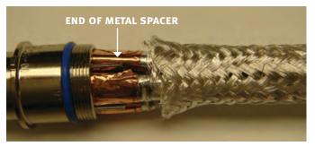
Figure 37: Trimming the braid
