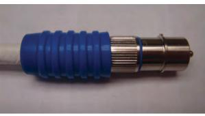
Figure 24: Seating the backshell
