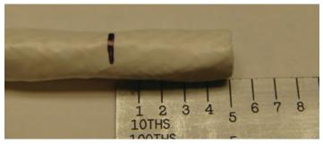
Figure 9: Marking the cable
