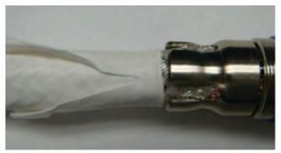
Figure 22: Returning the outer jacket
