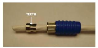
Figure 25: Sliding components onto the cable
