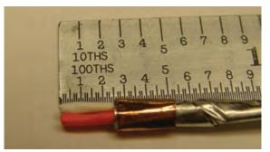
Figure 31: Removing the foil edge
