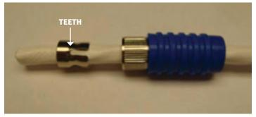
Figure 8: Sliding components onto the cable
