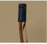
Figure 17: Inserting contacts into insulators
