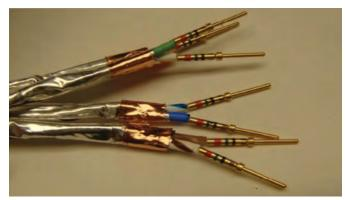
11. Using a blue insulator from the connector kit, insert the contact into an insulator with the solid colored wire in the hole on the left (Figure 17). Be sure to maintain a twist in each pair while inserting it into the insulator.
