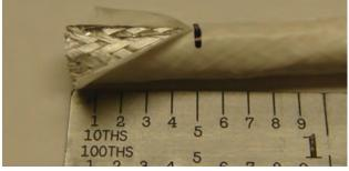
Figure 27: Slitting the cable jacket
