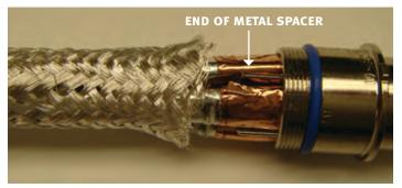
Figure 20: Trimming the braid
