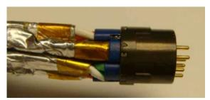
Figure 27: Pairs inserted into top insert
