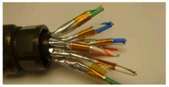
Figure 22: Removing the foil
