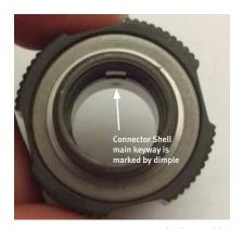
Figure 29: Inserting connector shell on cable
