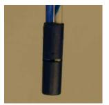
Figure 41: Inserting pair into insulator
