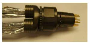
Figure 28: Top and bottom inserts together
