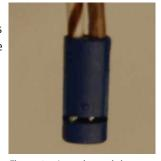
Figure 25: Inserting pair into plug insulator
