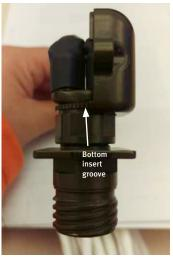
Figure 51: Attaching backshell
