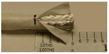
Figure 16: Slitting the cable jacket
