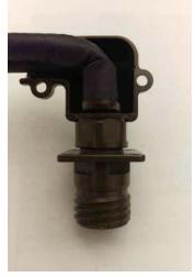
Figure 52: Attaching right-angle backshell
