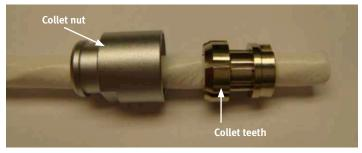
Figure 27: Attaching the collet and collet nut
