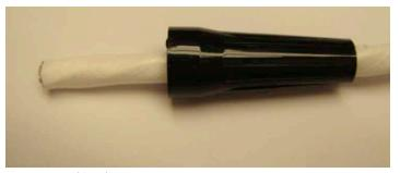
Figure 8: Attaching the connector cap
