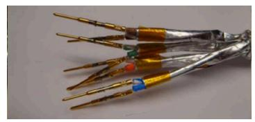
Figure 17: Stripping the pairs
