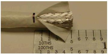
Figure 29: Slitting the cable jacket
