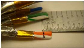
Figure 16: Marking each conductor
