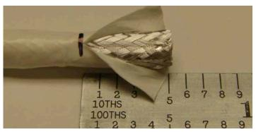
Figure 11: Slitting the cable jacket
