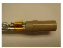
Figure 36: Inserting contacts into insulator
