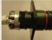
Figure 45:Trimming excess braid on plug
