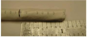
Figure 27: Marking the cable
