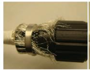
Figure 43: Attaching Band-It to plug
