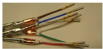
Figure 38: Stripping and crimping primaries
