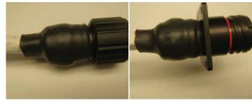
Figure 49: Shrinking tubing on plug Figure 50: Shrinking tubing on receptacle
