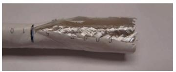
Figure 28: Slitting the cable jacket
