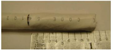
Figure 11: Marking the cable
