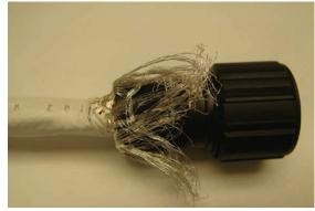
Figure 42: Returning the outer jacket
