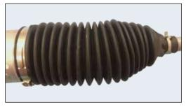
Venting prevents deformation, preserving the boot's structural integrity and reliably maintaining its "as-designed" protective function.
