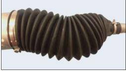
Sealed systems "trap" pressure differentials that cause boot deformation.
