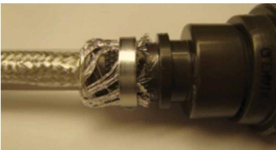
Figure 39: Attached Band-It® clamp
