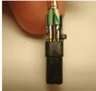
Figure 28: Attaching black rear insulator
