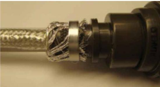
Figure 71: Attached Band-It® clamp
