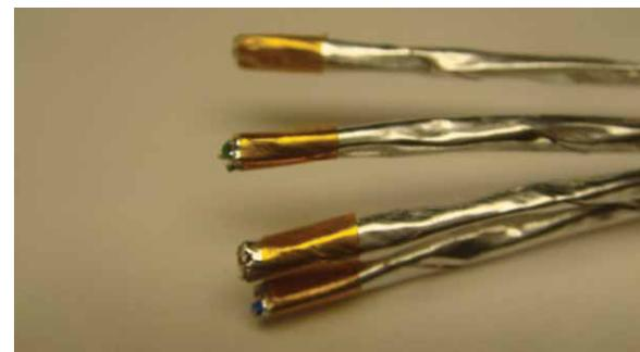
Figure 47: Taping each pair
