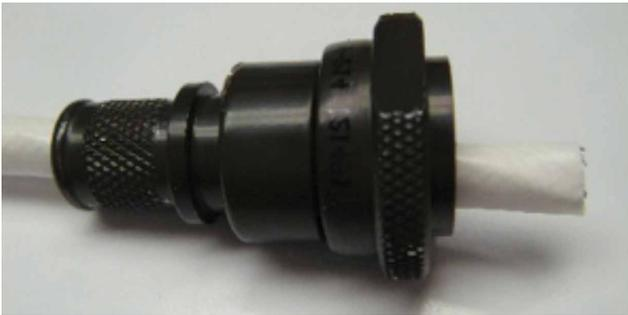
Figure 10: Inserting backshell on the cable
