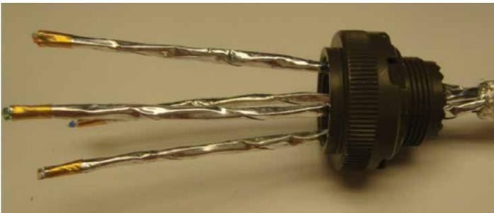
Figure 50: Positioning the grommet near the braid
