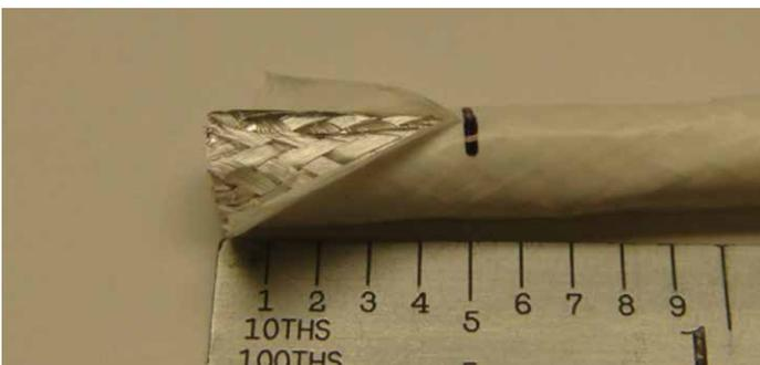
Figure 44: Slitting the cable jacket
