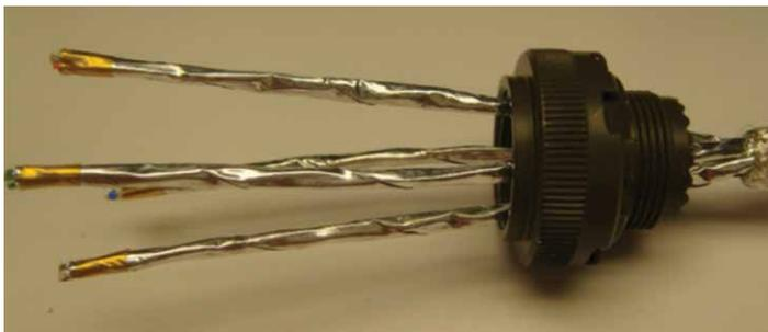
Figure 18: Positioning the grommet near the braid
