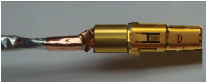
Figure 32: Positioning the ferrule
