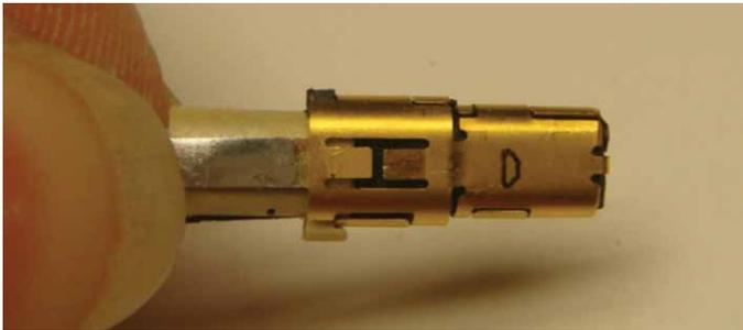
Figure 30: Locking outer body onto rear insulators
