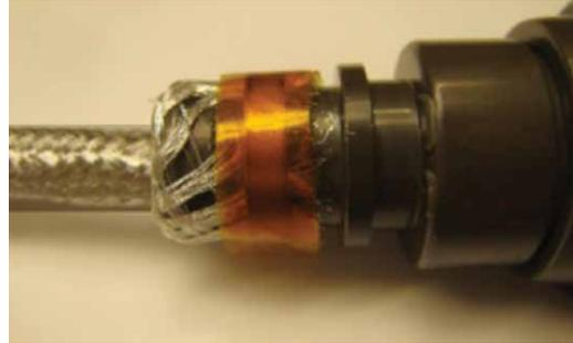
Figure 72: Wrapping Band-It® clamp
