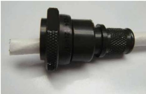
Figure 42: Inserting backshell on the cable
