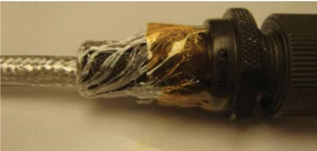
Figure 70: Returning braid to connector
