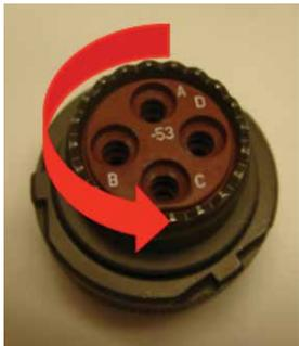
Figure 16: Inserting each pair into connector grommet
