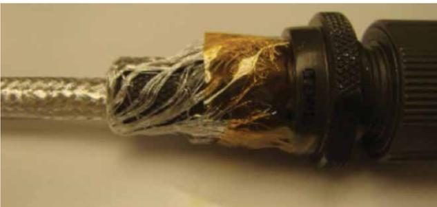
Figure 38: Returning braid to connector
