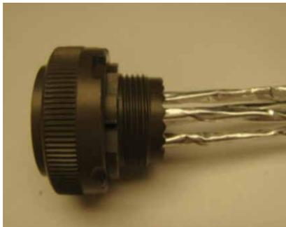
Figure 49: Pairs inserted in connector grommet
