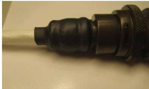
Figure 41: Shrinking tubing to backshell
