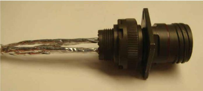
Figure 69: Connecting the grommet to the receptacle
