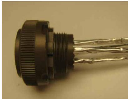
Figure 17: Pairs inserted in connector grommet
