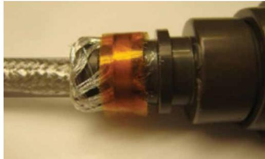
Figure 40: Wrapping Band-It® clamp
