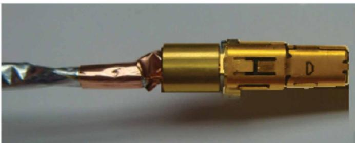
Figure 32: Positioning the ferrule
