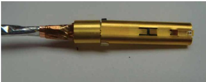
Figure 64: Positioning the ferrule
