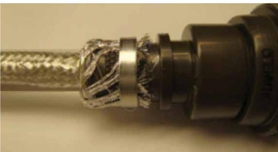
Figure 71: Attached Band-It® clamp
