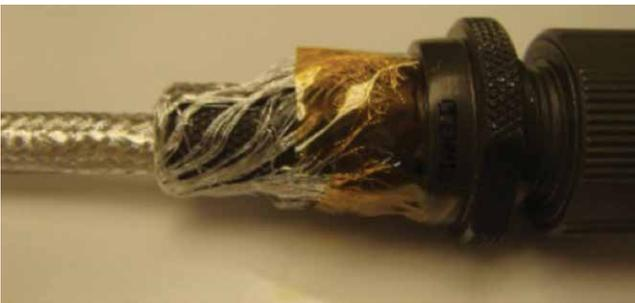
Figure 38: Returning braid to connector
