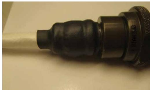
Figure 73: Shrinking tubing over backshell
