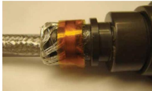
Figure 72: Wrapping Band-It® clamp
