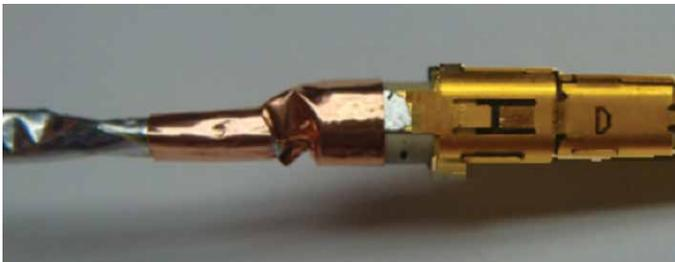
Figure 31: Taping the outer body ears
