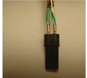
Figure 58: Soldering the twisted pair
