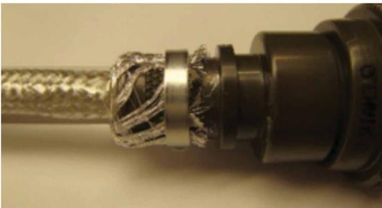
Figure 39: Attached Band-It® clamp
