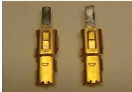
Figure 27: Tinning ears of outer body
