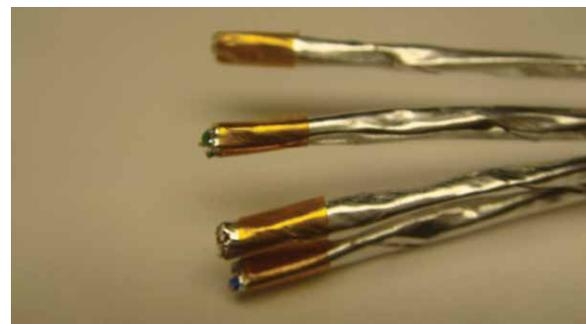
Figure 47: Taping each pair
