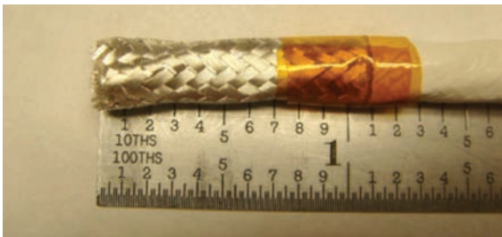
Figure 6: Wrapping the tape
