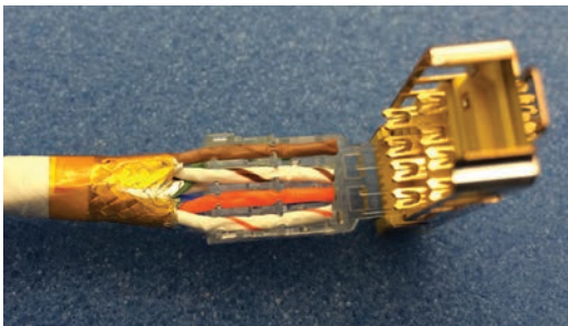
Figure 12: Wires inserted in position in top row
