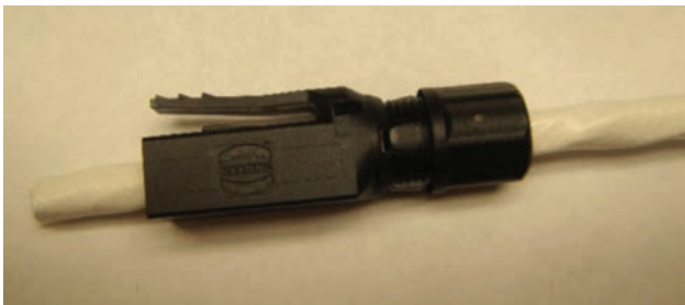
Figure 5: Attaching the labels, sleeving and black housing
