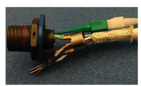
Figure 38: Inserting the wired contact in connector
