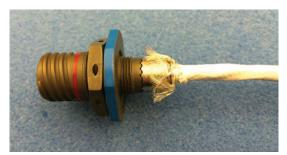
Figure 42: Trimming the excess braid material
