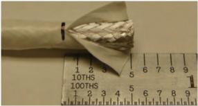
Figure 30: Slitting the cable jacket
