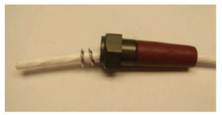
Figure 11: Sliding the backshell onto the cable
