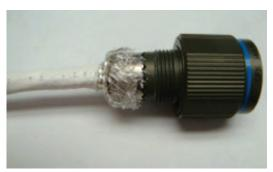
Figure 25: Trimming the excess braid material
