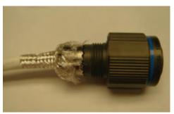
Figure 23: Folding the braid over the backshell
