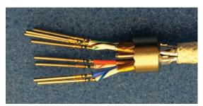
Figure 37: Inserting pairs through the metal follower
