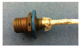
Figure 40: Folding the braid over the backshell
