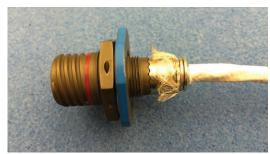
Figure 43: Placing the washers near the connector
