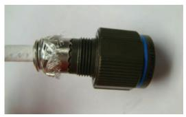
Figure 26: Placing the washers near the connector
