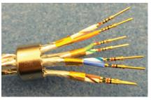
Figure 20: Inserting pairs through the metal follower
