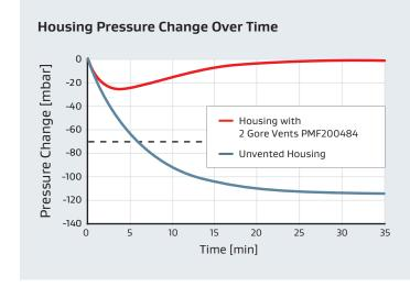
Temperatures inside the Moon Light's housing can reach 60 °C, and can drop to 20 °C causing extreme pressure differentials. Without a vent, the pressure can reach 115 mbar, which eventually causes the seals to leak and water and contaminants to enter the housing. Using a GORE® Protective Vent provides continuous airflow to equalize pressure rapidly and prevent contamination.
