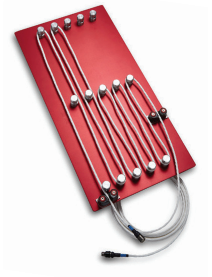
Figure 15: Cable Routing Simulator
